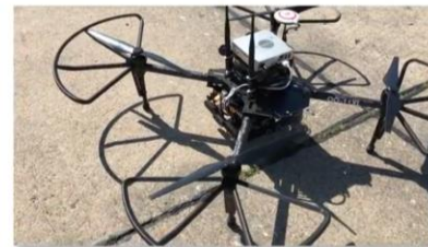
DJI Matrice 100 DJI Manifold Wi-Fi (.11n, 2 monopole antennas) RocketM5 (2 cloverleaf antennas)
