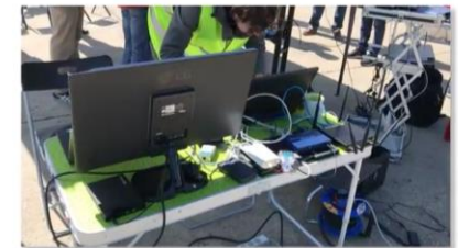
Mini-PC gateway/router batteries, switch, 4G uplink Wi-Fi (.11n, 2 monopole antennas) RocketM5 (2 cloverleaf antennas)
